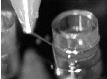
Figure 2: Capture of the wire bonder head in movement during the micro coil winding process.
