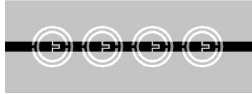
Figure 6. Microstrip line (black) with CSRRs etched in ground plane (gray). Capacitive gaps have been etched on the strip to obtain a left-handed passband. Adopted from [20].
