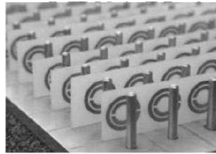
Figure 2. The array of split-ring resonators plus wire assemblies used for the experiment. Adopted from [11].
