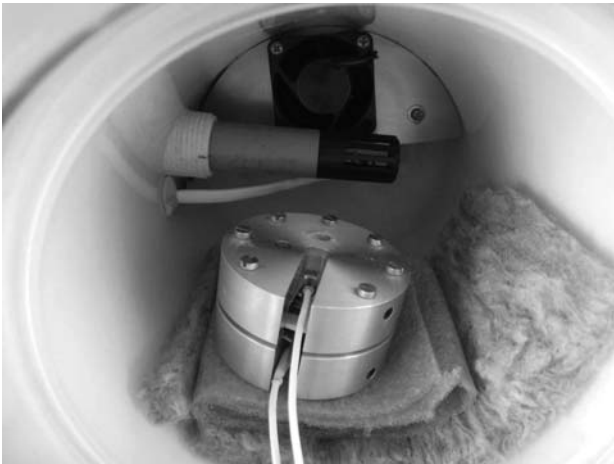
Figure 3. The external reference capacitor in an oven encapsulating an AI block with vibration dumping.
