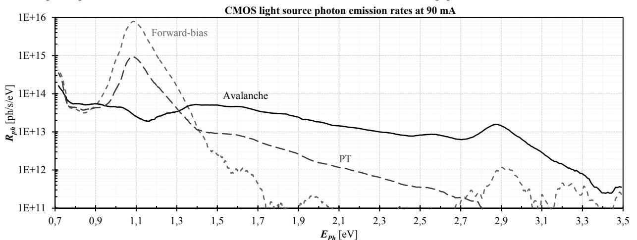
Figure 3: Calculated photon emission rate spectra of the avalanche, forward-biased and PT CMOS light sources.
