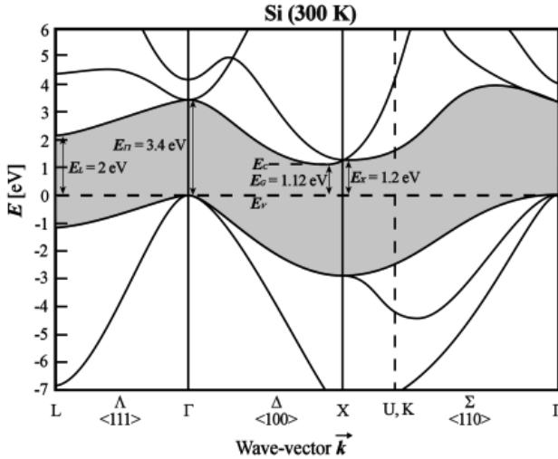
Figure 4: Si energy band diagram at 300 K [10].
