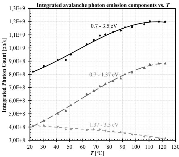
Figure 9: Integrated avalanche spectral components against temperature.
