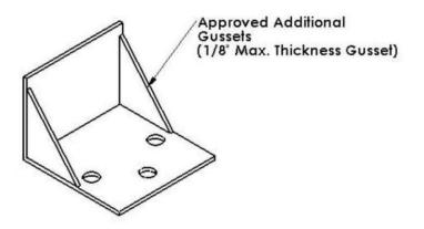
Upper Link Double Shear Mount (Chassis Side)
