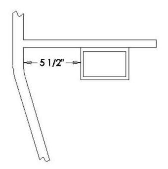
Note: The measurement for the battery box offset will be taken at the point closest to the crossmember, from the inside of the framerail to the otside of the battery box.
