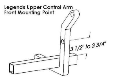
3 1/2" to 3 3/4" (from the top of the frame to the center of the pick-up point holes)
