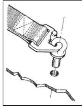
It is recommended that the anchorage points of the vehicle manufacturer be utilised wherever possible in respect to mounting of the safety harness. Any drilled anchor point must be properly reinforced to accept the load which will be applied thereto during a crash.
