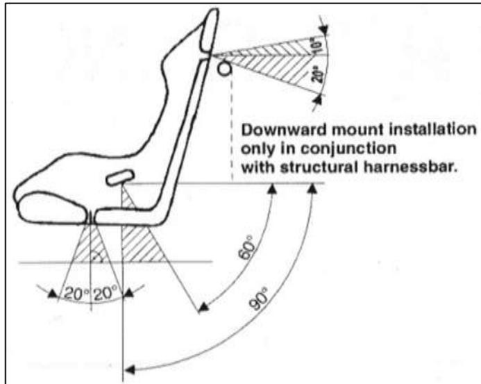
Never run the shoulder straps downwards from the backrest slots without a strap support bar which can withstand the load applied to it during a crash. The seat backrest is not designed to accommodate this load and may collapse in the event of an accident, thereby greatly increasing forward movement of the occupant which can cause serious injury or death.
