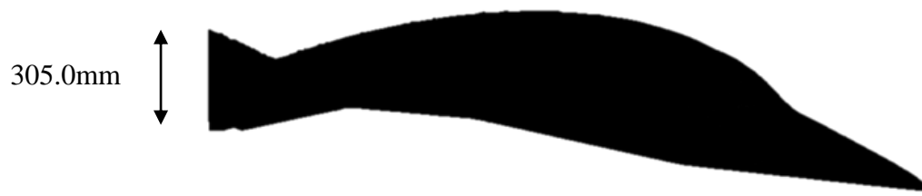
Left hand and right hand side pod floor. Material: marine ply wood, 6mm thick
