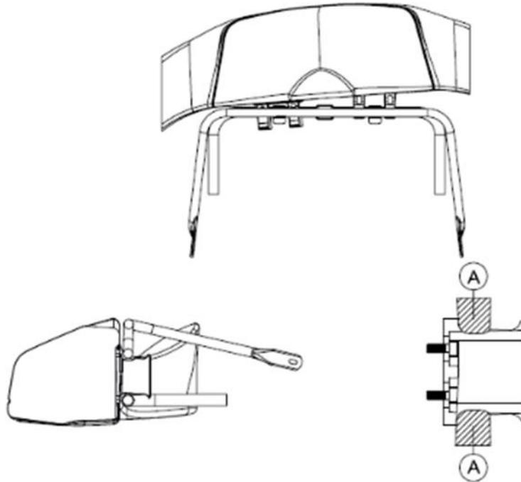
Partial dislodgement – One side of the bumper is in the incorrect position
