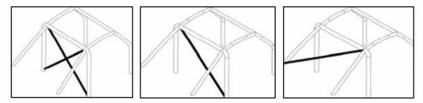
The above sketches are courtesy of the FIA web site and depict the acceptable style of cross bracing (the black pipe) for roll cages. Obviously these drawings assume proper base plates and welding.
