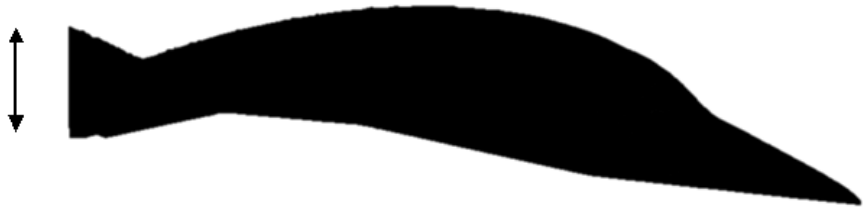
Left hand and right hand side pod floor. Material: marine ply wood, 6mm thick
