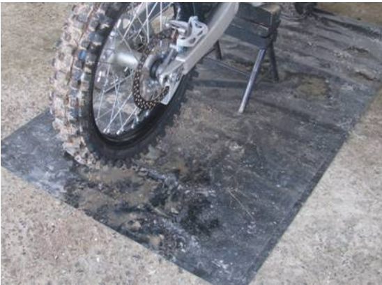
Above: Ordinary plastic sheeting does not provide proper protection when used as an “enviro mat”. It has no absorption qualities. Fluids form puddles and will eventually run off and pollute soil and/or water sources. Newspapers, cardboard boxes, etc. also do not address proper pollution control.
