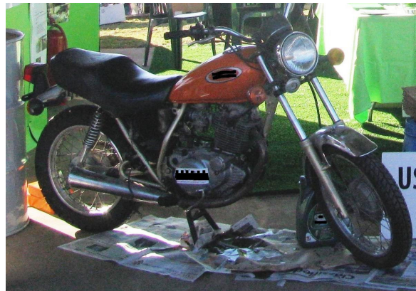
Above: Ordinary plastic sheeting does not provide proper protection when used as an “enviro mat”. It has no absorption qualities. Fluids form puddles and will eventually run off and pollute soil and/or water sources. Newspapers, cardboard boxes, etc. also do not address proper pollution control.
