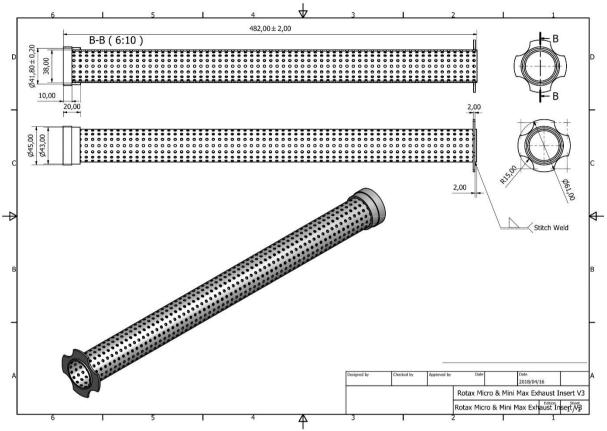
This insert must be wrapped first with stainless steel mesh (wire 0.23mm and 0.33mm square openings) 455x130mm secured by 5 stainless steel pull-ties, positioned approximately 15mm from each end and equally spaced at approximately 106mm intervals. An original Rotax exhaust matt cut to 160mm x 480mm and installed into the original exhaust with the correct baffle for Micro and Mini Max.
