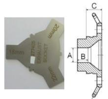
Fit the template (Micro MAX "18 mm") as far as possible into the exhaust socket (without gasket, carbon deposits removed). There has to be a constant crack light between the profile of the exhaust socket and the profile of the template.
