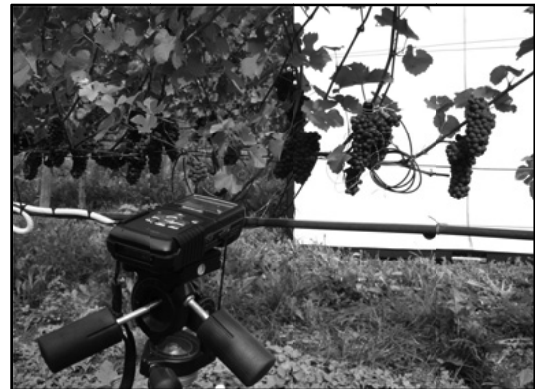
Figure 2: Thermal imager set up for measurements of grape bunch temperatures.
