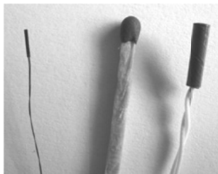
Figure 1: Thin (left) and thick (right) type thermocouples that can be used in grape berry temperature assessment.
