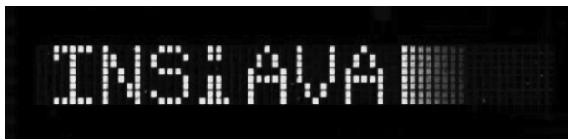
Figure 4: Image formed on the all-CMOS microdisplay clearly showing the illuminated pixels in contrast to the true-black (off) pixels [10].
