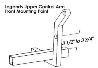
3  $1/2^{\circ}$  to 3  $3/4^{\circ}$  (from the top of the frame to the center of the pick-up point holes)
