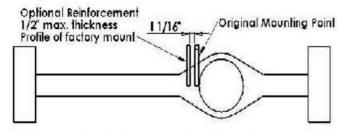
(This reinforcement will secure the opposite side of the rod end of the upper link)
